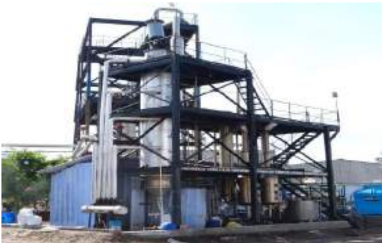
Agitated Thin Film Dryer Machine (A.T.F.D) at Tamil Nadu Co-operative Textile Processing Mills
