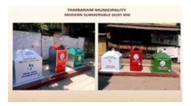
**11.34** Each semi-submersible bins has the coloured and illustrated half above the ground level and remaining portion embedded in the ground and has a capacity of 700 Kgs. The unique design allows for natural compaction due to gravity and less odor. The bins will be lifted twice a week using a specially designed crane. Within a short period of time these bins have captured the imagination of the local people and have become their favorite mode of disposal.
